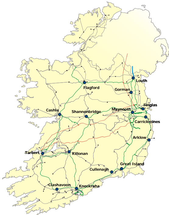
Figure 7-1 220 kV Stations Studied for Generation Capability
